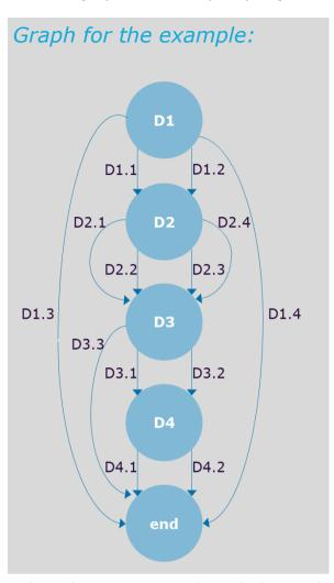
A logical test case runs through the graph from beginning to end, forming a chain of test situations. The graph also gives insight into the minimum number of test cases necessary to cover all the test situations. This is determined by the maximum number of parallel lines in the graph (in this example this is 6).
