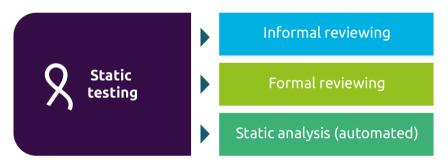
Static code analysis is a collection of algorithms and techniques used to analyze source code in order to automatically find (potential) faults, vulnerabilities or poor coding practices. An example of a result of static testing are compiler warnings (which can be useful for finding coding errors), but static code analysis with more sophisticated tools takes that idea a step further to find faults that are traditionally found by dynamic testing.
