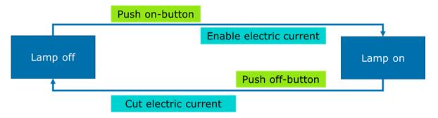
Pictured above is an example of a simple state transition diagram. Our example system is a lamp. The lamp can be off or on. If the on-button is pushed, the electric current is enabled and the lamp is turned on. If the off-button is pushed, the electric current is cut and the lamp is turned off.
